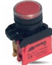
SW-AW3475 22mm LEDLİ IŞIKLI YAYLI BUTON STOP - 110-240V AC / 1NC 22mm LED ILLUMINATED SPRING-RETURN STOP-PUSH BUTTON 110-240V AC /1NC
