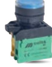
SW-AW3675 22mm LED IŞIKLI YAYLI BUTON 110-240V AC / 1NO 22mm LED ILLUMINATED SPRING-RETURN START-PUSH BUTTON 110-240V AC /1NO
