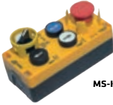
MS-KYD05 ACİL STOP BUTON +2 OKLU BUTON ORTAK OKLU (1NO) SEÇİCİ BUTON (2NO-1NC) CONTROL BOX WITH EMERGENCY STOP, DUAL ARROW BUTTONS, SHARED 1NO ARROW, AND 2NO+1NC SELECTOR SWITCH
