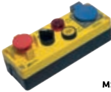
MS-KY5-24 KORUMALI ACİL STOP BUTON (1NC) LAMBA VAVİEN (1NO) 24V KATTA LED (1NO) ALARM BUTON 16A KAPAKLI PRİZ
