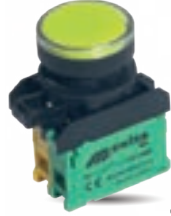
SW-AW3575-24 22mm LED IŞIKLI YAYLI BUTON 10-30V DC / 1NO 22mm LED ILLUMINATED SPRING-RETURN START-PUSH BUTTON 10-30V DC /1NO
